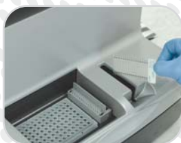
Sample Tube, Tip and ScreenTape placed in the TapeStation
